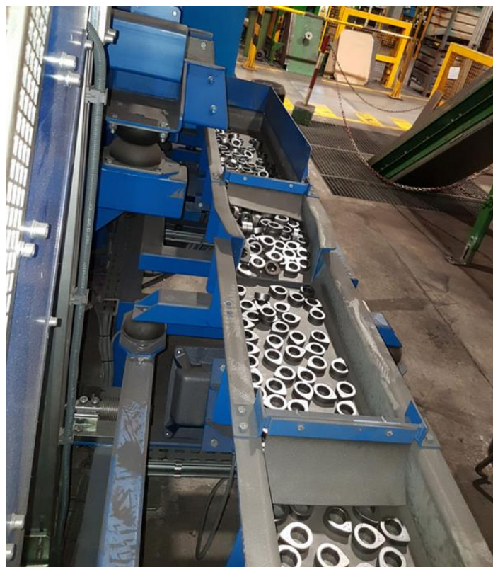
Fig. 4. Technological process of transporting parts using a vibrating conveyor
